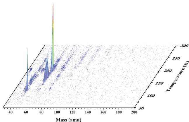
**Figure 2.** Reflectron time-of-flight (ReTOF) mass spectra as a function of temperature of the newly formed products subliming into the gas phase from radiation processed methanol ice obtained at photoionization energy of 10.49 eV. The absence of signal at mass-to-charge larger than  $m/z$  100 verifies the absence of any glycerol dimers subliming.
